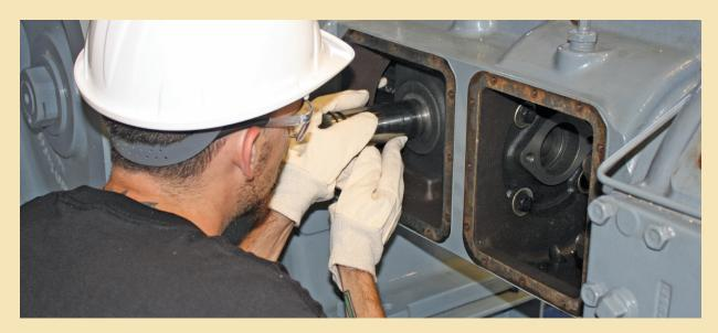
The 40-hour Advanced Reciprocal Compressor training class covers every level of compressors: Basic knowledge of compressors and how they work, disassembly and problem diagnosis, and reassembly to exact specifications. Before millwrights are cleared to take the advanced compressor course, they must display proficiency in the basic 40-hour Reciprocal Compressor Training Class.
