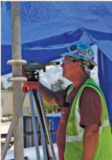
Mike Stewart shooting elevations with an optical micrometer
